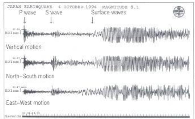
d A seismogram showing the three different waves.
