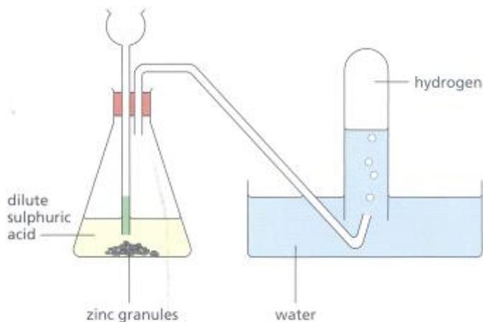
Figure 16.11 The laboratory preparation of hydrogen gas.
