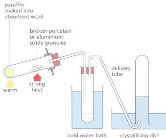
Figure 12.13 The cracking of an alkane in the laboratory.
