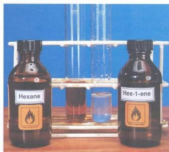
Figure 12.15 The alkene decolorises bromine in 1,1,1-trichloroethane.
