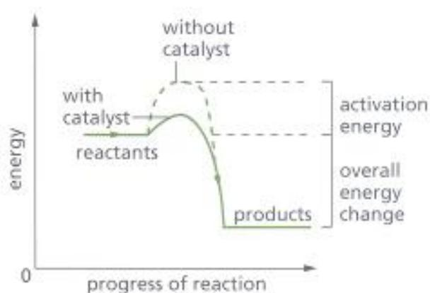
Figure 11.10 Energy level diagram showing activation energy.
