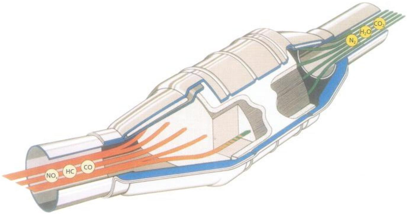
b A section through a catalytic converter.
