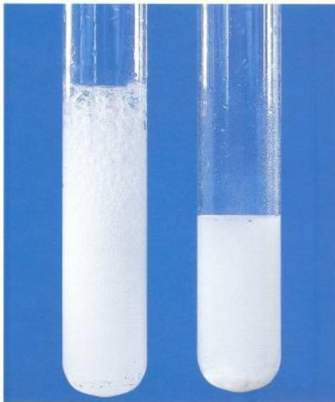
Figure 11.2 The powdered limestone (left) reacts faster with the acid than the limestone in the form of lumps.
