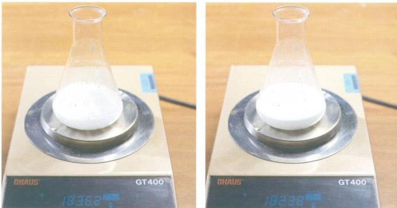
Figure 11.3 After 60 seconds the mass has fallen by 1.24 g.
