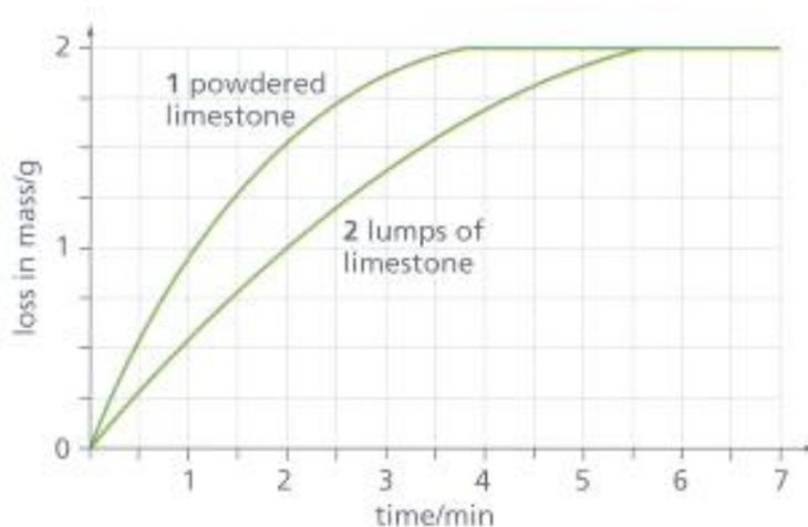
Figure 11.4 Sample results for the limestone/acid experiment.
