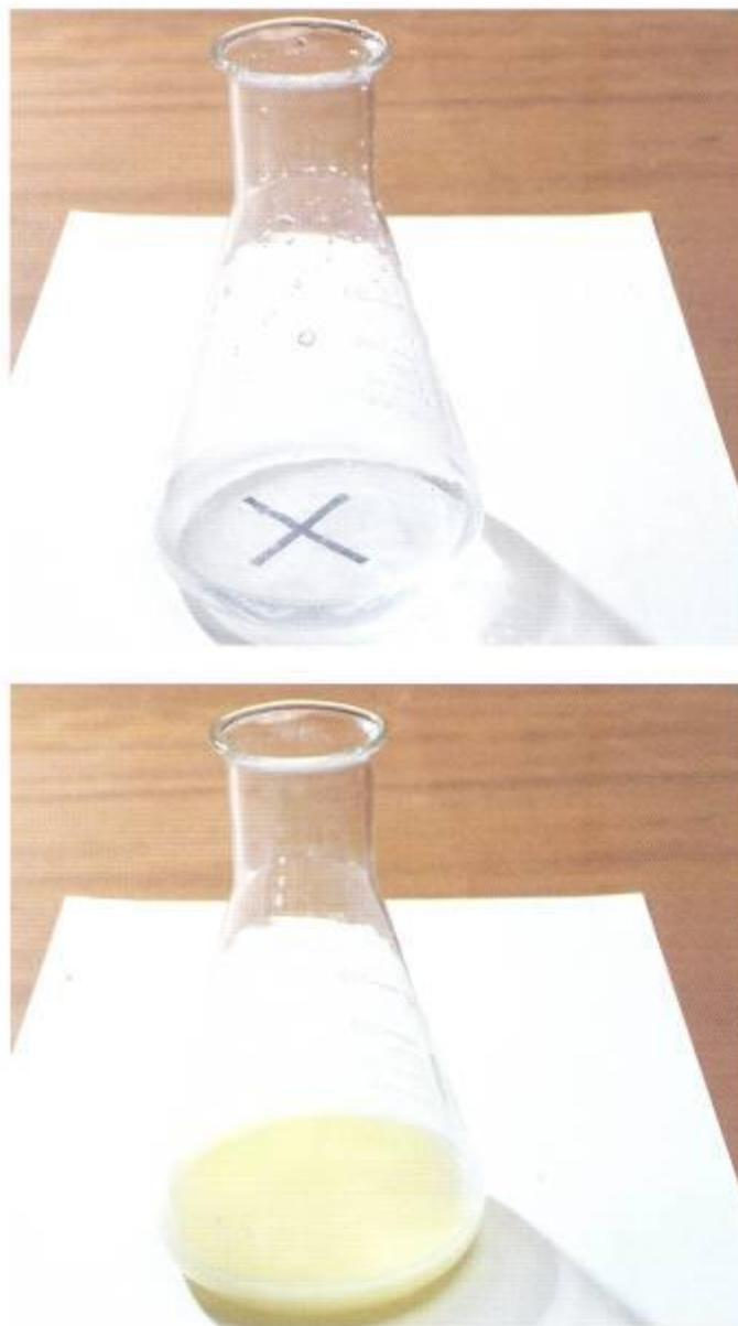
Figure 11.6 The precipitate of sulphur obscures the cross.
