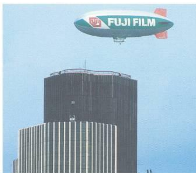
Figure 10.12 Helium is used to fill this airship as it has a low density and is unreactive.
